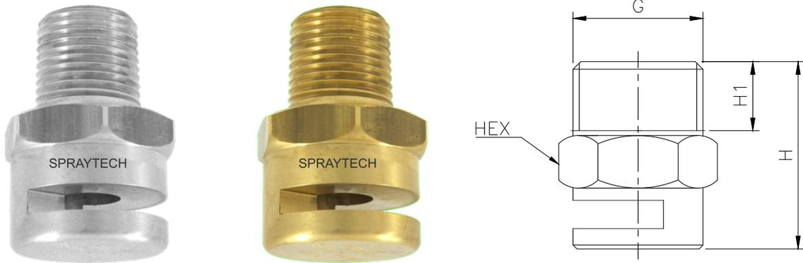
Spraytech' s Curtain Nozzles are sprinklers intended for protection of windows, walls and roofs against exposure fires. It generates uniform flat fan spray pattern and are installed on manual or automatic deluge systems. Window Curtain Nozzles are available in SS and Brass material of construction with different flow rates/ K-factors.
