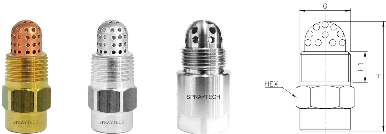
Spraytech's High Velocity Water Spray Nozzles are specially designed for use in fixed water spray or deluge system for the fire protection application. It has internal vane design to generate uniform solid/Full cone spray pattern and dense core of high velocity water spray for efficient fire control.
